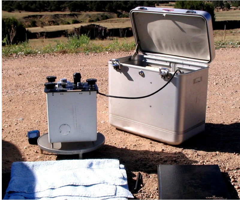
Figure 8 Typical gravity station measurement showing the gravity meter, GPS receiver and field notebook. The towel is for an old man's knees.
